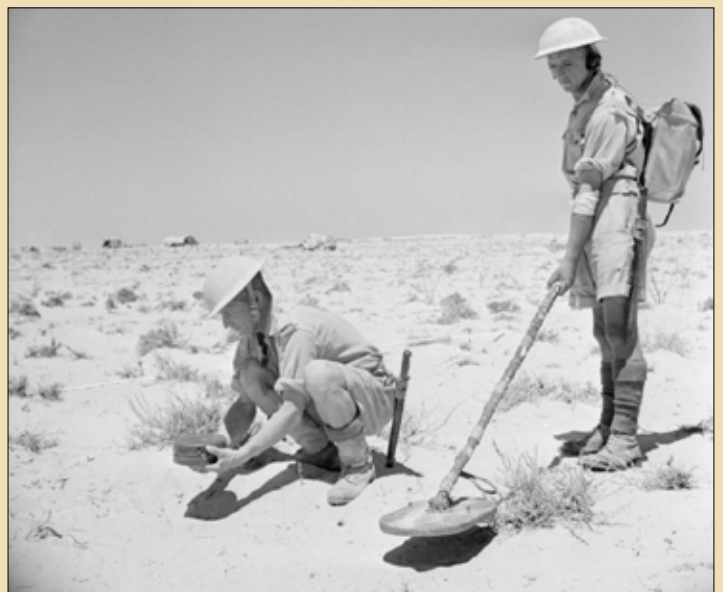
British sappers using a MK1 mine detector in El Alamein, Egypt during World War II
