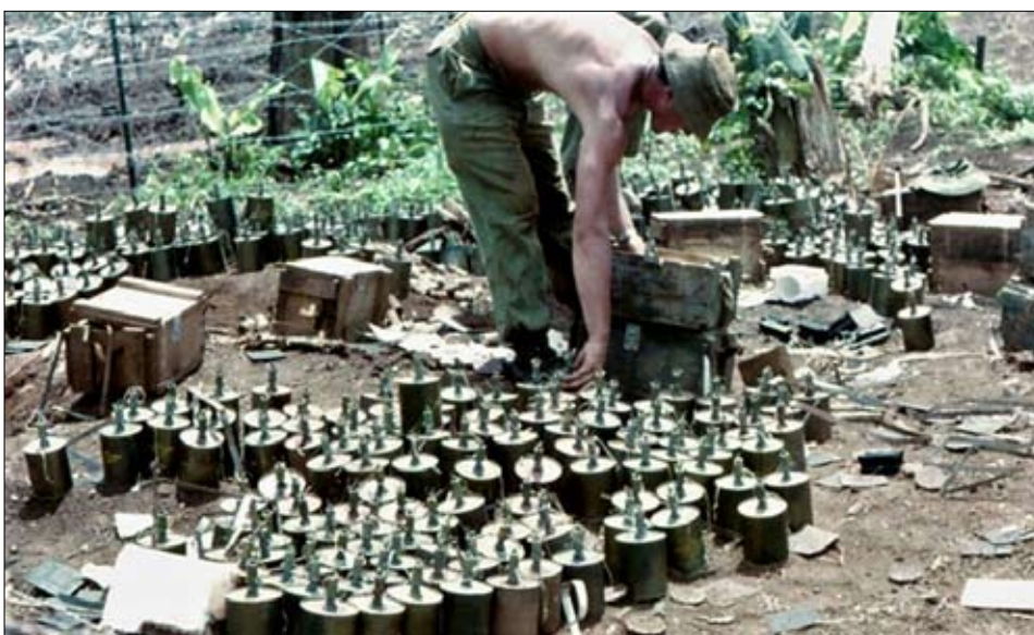
TOP: Boxes of M-16 mines nearby the minefield, ready for unpacking. ABOVE: M-16 mines unpacked, with fuzes fitted, ready for laying.
