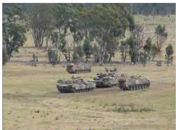
Above: Unserviceable Abrams MBT being recovered by an M88 Hercules Armoured Recovery Vehicle, with support from M113 APC and Ambulance.
