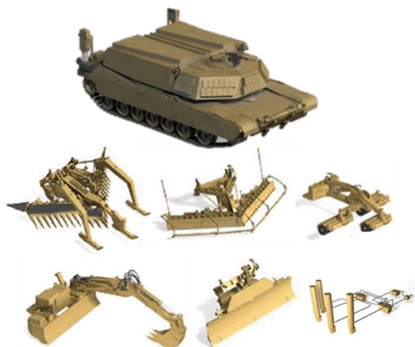
M1150 Assault Breacher Vehicle Front End Equipment from Pearsons Engineering Limited
