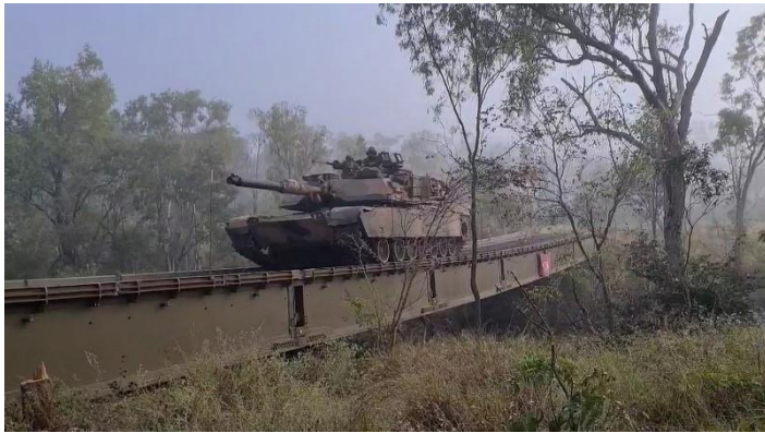
An M1A1 from 2 CAV crosses a Dry Support Bridge emplaced by 3 CER on Ex Brolga Run
