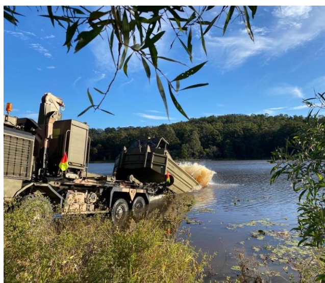
BEPB being launched off a HX77 in to the Enoggera Dam at GAL BKS
