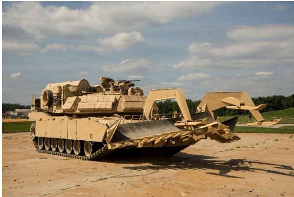
M1150 Assault Breacher Vehicle (ABV) with Full-Width Mine Plough (raised position).
