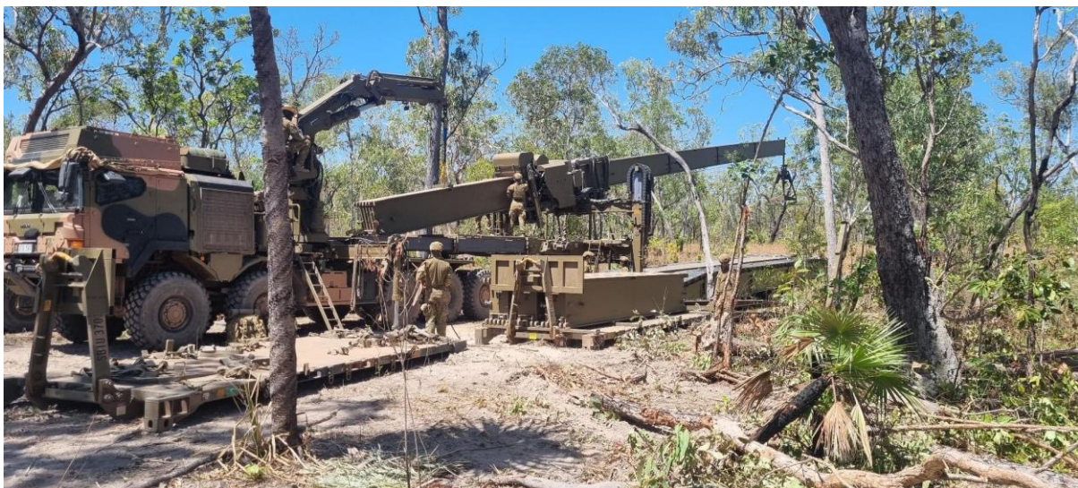
Specialist Troop deploying the Dry Support Bridge to enable lines of communication within Mount Bunday Training Area
