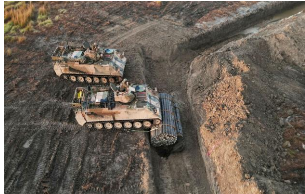
Sappers from 7 CE SQN drop a fascine in an anti-tank ditch during 7 BDE combined arms training in Shoalwater Bay.
