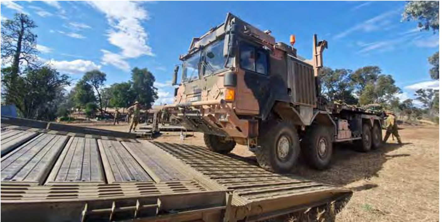
An HX-77 heavy vehicle drives onto a Medium Girder Bridge during Ex SAPPER SPAN in Gayndah, QLD.
