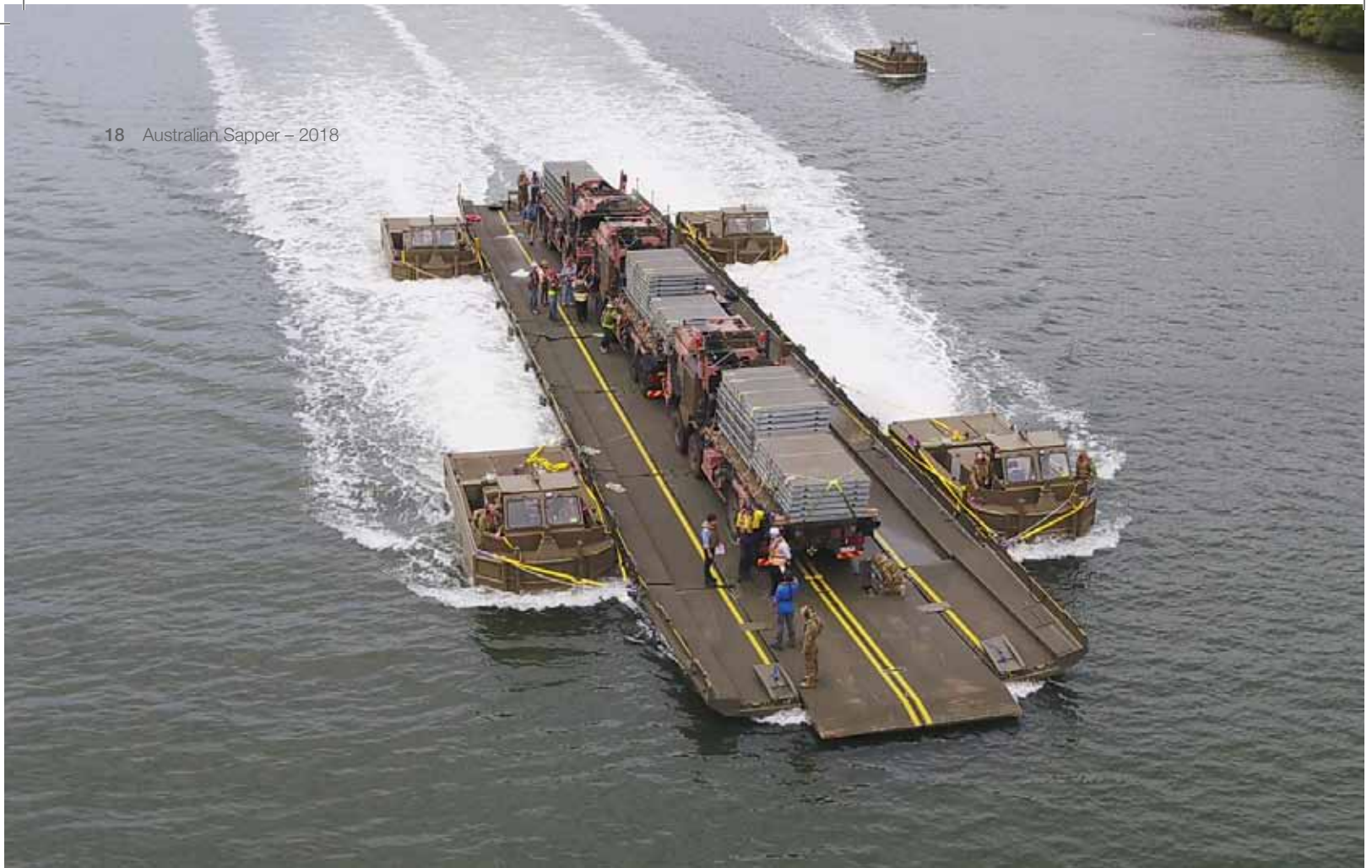
The Improved Ribbon Bridge is tested in the 7 Bay Raft configuration (100t capacity) during introduction into service testing November 2018, as part of L155.
