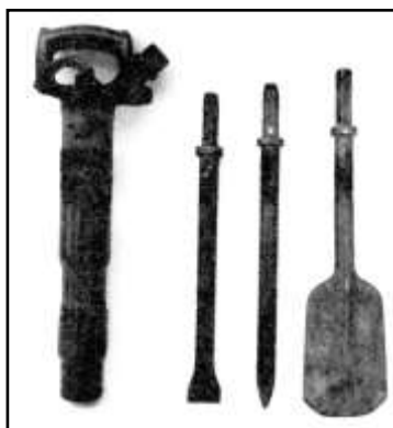
The Light Pick (left) and the Heavy Breaker (Below) were powered by an Ingersoll - Rand compressor.
