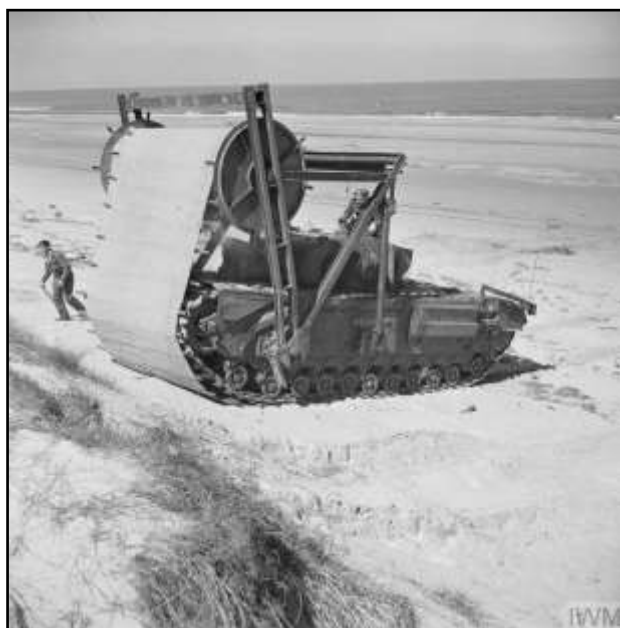
Bobbin tank laying trackway in training.
