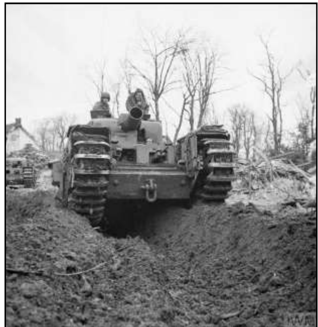
The Churchill AVRE (Armoured Vehicle Royal Engineer) was a modified Churchill tank fitted with a Petard spigot mortar, designed primarily to demolish steel and concrete structures, such as bunkers and gun emplacements. Specialised equipment could be added to the AVRE to enable it to perform other tasks.
